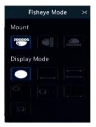
Three mounting modes are available: ceiling, wall, desktop. Ceiling and desktop mounting modes use the same dewarping method.
