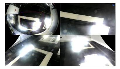
On a PTZ image, drag the mouse to rotate the image or use the scroll wheel to zoom in or out. A box appears on the fisheye image as the image rotates, and as you drag the box or move the scroll wheel on the fisheye image, the corresponding PTZ image rotates or zooms in or out as well.
